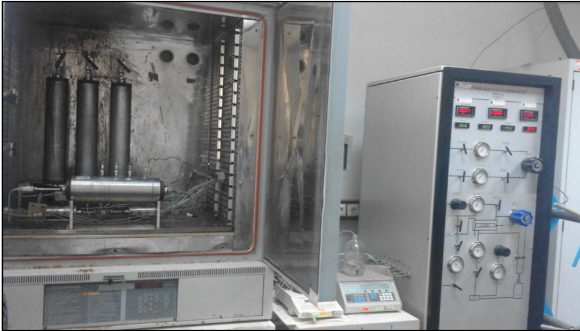
Figure (B.3) : appareil de colmatage(DAFFM).
