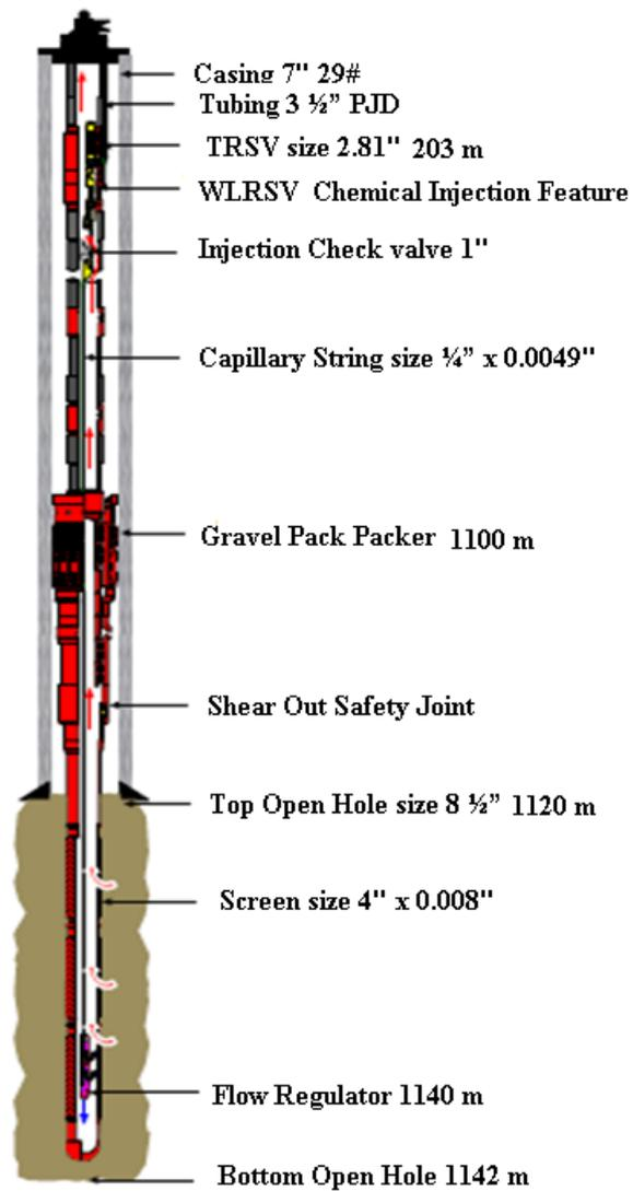
(Figure III.16 :) l'installation de tube capillaire [22]
