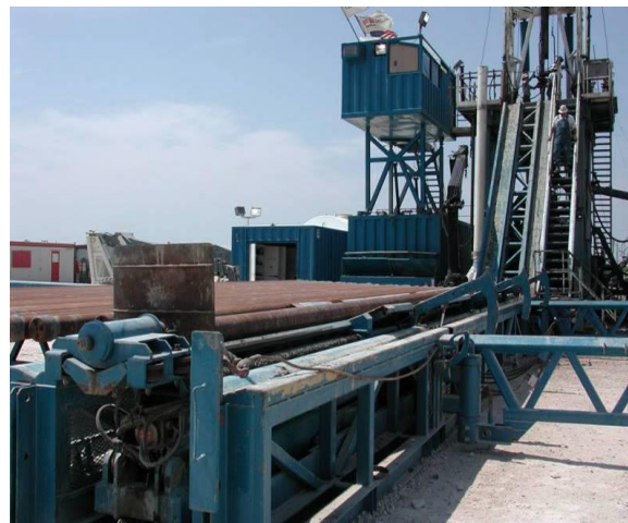
Figure I.8.-Power catwalk for DwC
