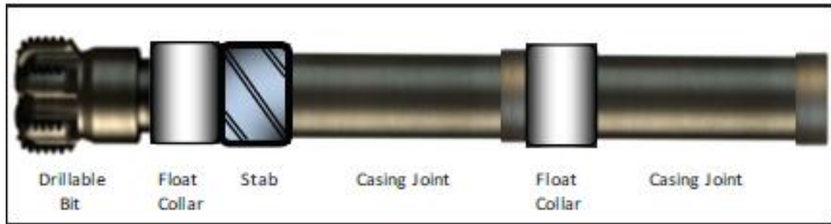
Figure.III.2—BHA designed for CwD job in Fields A and B (no stab needed and only 1 float collar).
