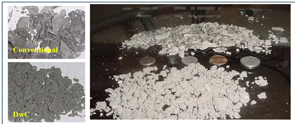
Figure II.7.-Cutting comparison between DwC and conventional drilling
