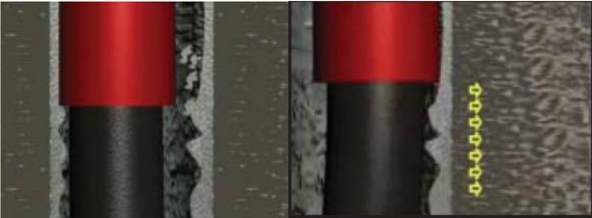
Figure I.3. The casing is forced against the bore wall and cuttings are smeared into the formation.
