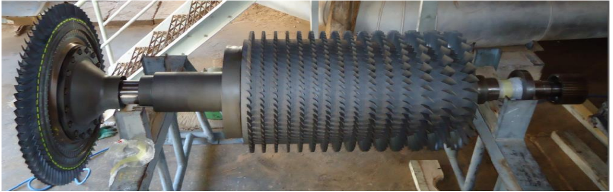
Figure I-2: Ensemble rotor compresseur /roue turbine HP.
