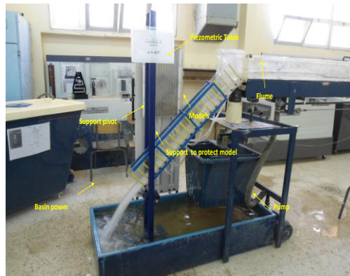
Photo 1: Experimental device (Gafsi and Benamamar, 2013a, b)
