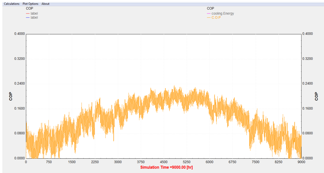
Figure 3.16: variation de COP d'une machine a absorption (Performance Map Collector)
