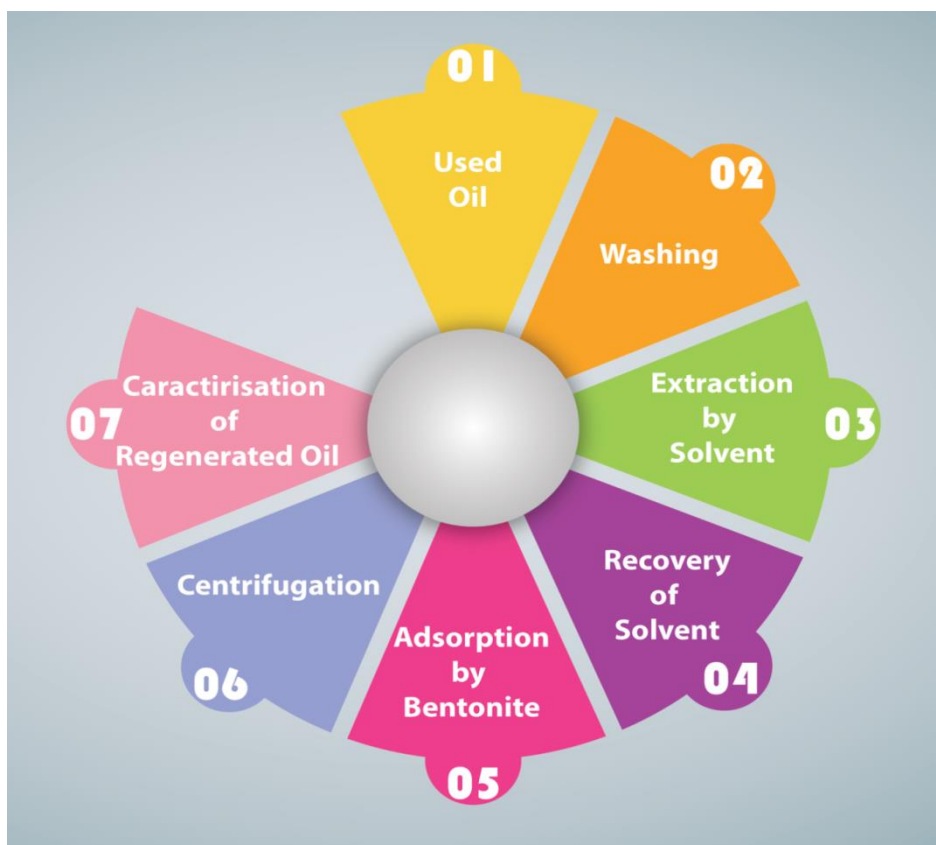
Figure II.1. Scheme which combines the different steps of the treatment procedure
