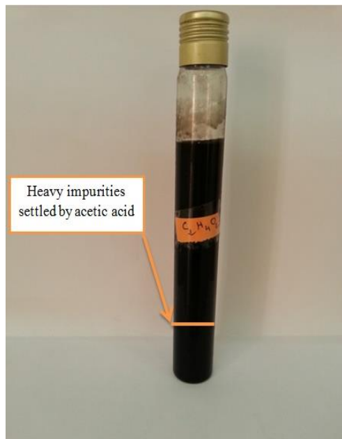
Figure III.2. Sludge formation using acetic acid
