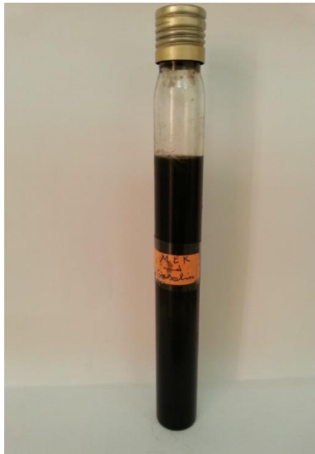
Figure III.6. MEK separates the sludge from the oil
