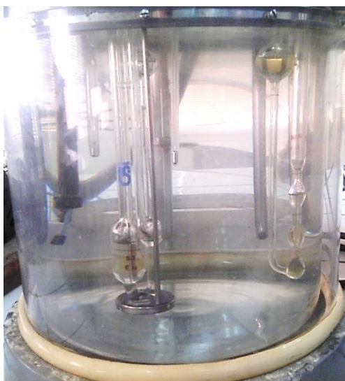
Figure II.12. Position of viscometer in bath water
