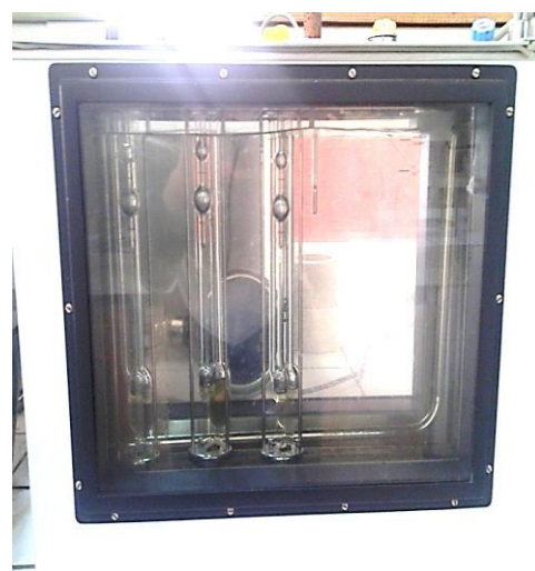
Figure II.13. Position of viscometer in bath oil
