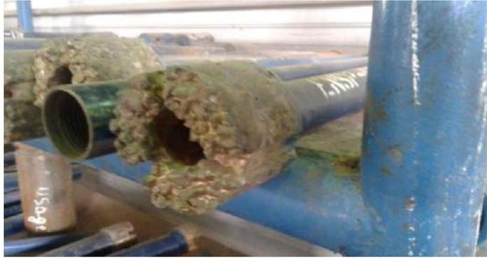
**Figure III-6: OUTIL DE MILLING**
