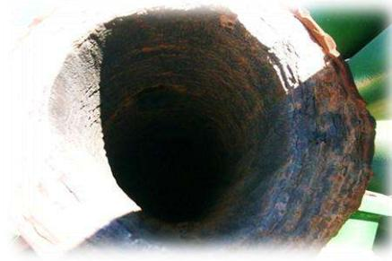
**Figure II-3 : DEPOTS DE  $\text{CaSO}_4$  DANS UNE PIPE DE PETROLE [16]**
