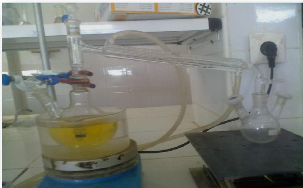
Figure III.13: Montage de distillation
