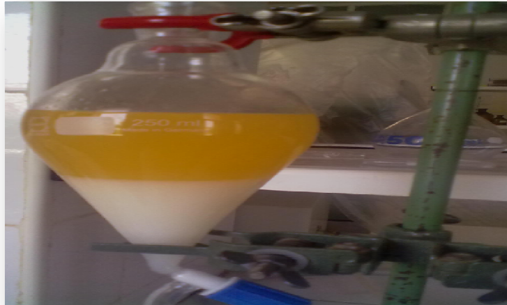
Figure III.12: Photo de lavage du biodiesel
