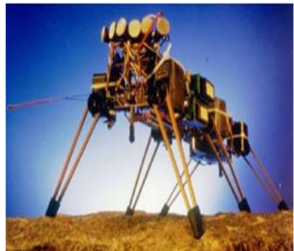
Fig. I.8: Genghis, developed by Rodney Brooks at MIT in the early 1990s
