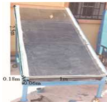
Figure 4.18: Photograph of the solar collector.
