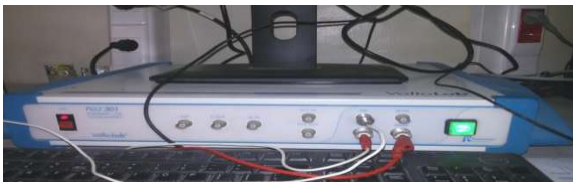
Figure .II.5 : potentiostat Voltalab 40(PGZ 301) (Radiometer Analytical)
