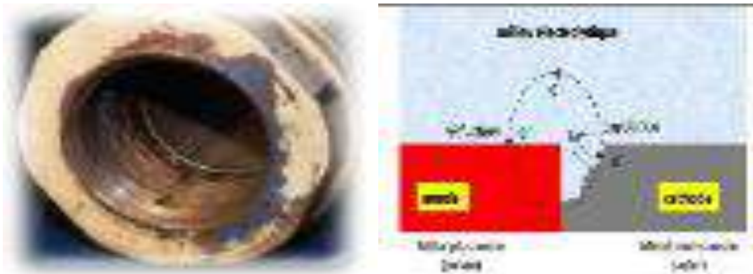
Figure(I.2): la corrosion galvanique
