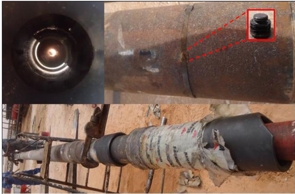
Figure III.6 : Le PBR (Polish Bore Receptacle) (2)
