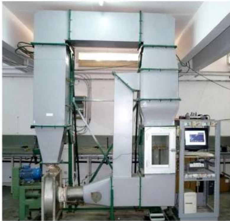
Figure 3.5.a: Picture of the experimental laboratory LETTM dryer (Drying loop).
