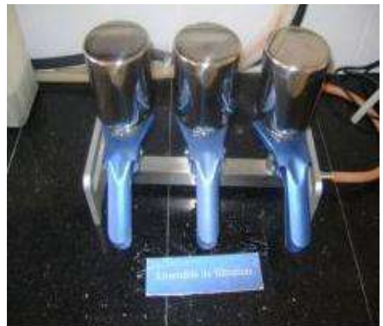
Figure N 26 rampe de filtration
