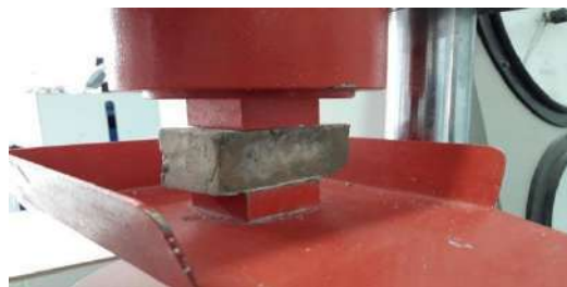
Photo III.3. Essai de compression.
