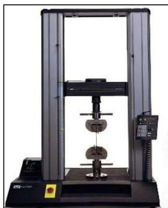
**Figure (II.10) :** Machine de traction.
