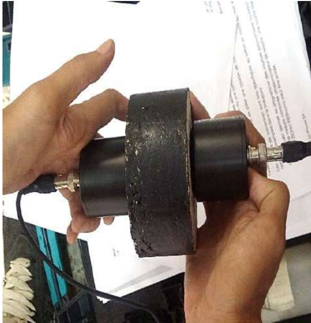
Figure VI.4. The direct ultrasonic test “fly time measurement”
