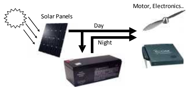
Figure.1 Solar airplane basic principle
