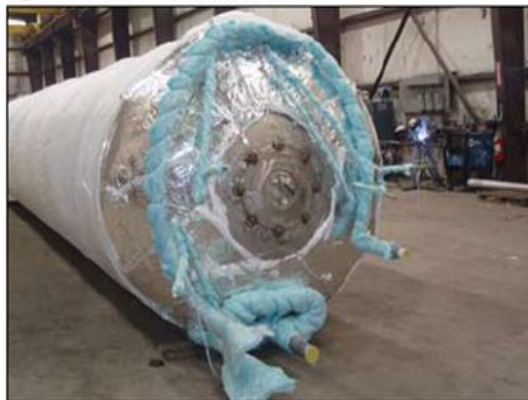
Figure 5-3. Inner Vessel with SI Insulation
