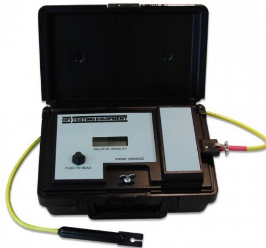
Figure (I-5): Emulsion Stability Tester. [10].
