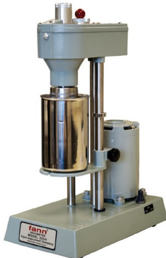
Figure (I-2): Direct indicating viscometer (6 speed). [6]
