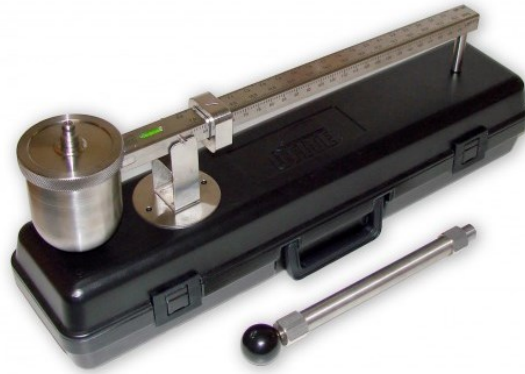
Figure (I-1): Drilling fluid balance used to measure fluid density. [10]
