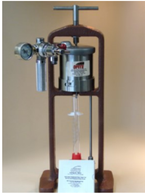
Figure (I-3): API low-temperature, low-pressure filter press [6].
