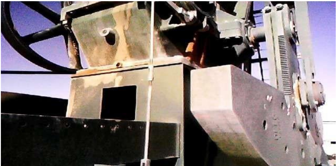
Figure III.24 : LE CONTREPOITS (MODIFIE) [6]
