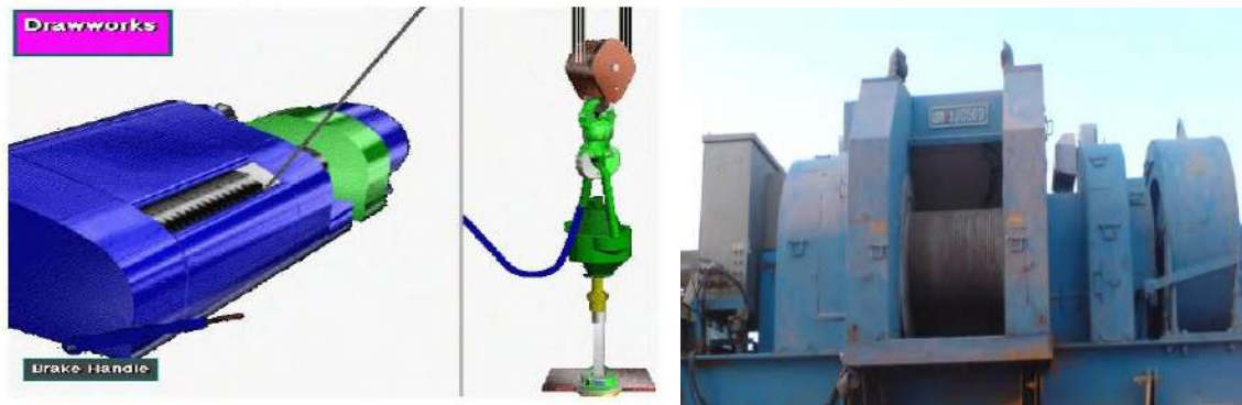
Figure I.7 Treuil de forage
