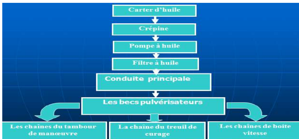
Figure I.14 : Circuit de lubrification. [16]
