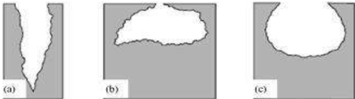
Figure I.4: Pitting forms (a) deep cavity (b) cavernous cavity (c) hemispheric [11].
