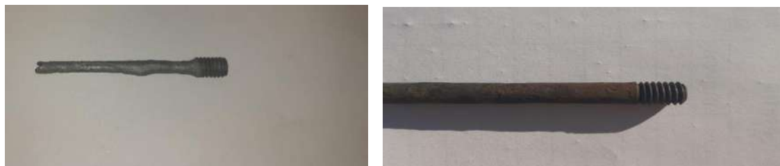
(1) Severe v corrosion
