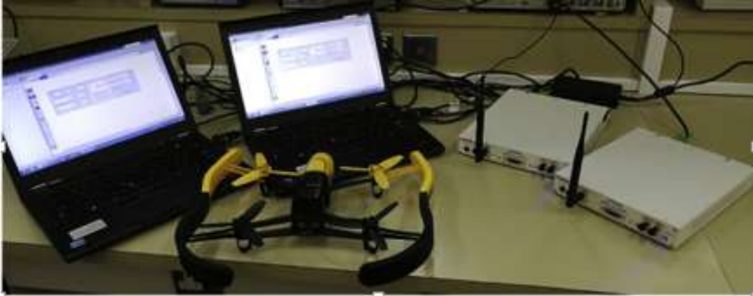
FIGURE 5.1: Experimental setup for the RF database development. The Bebop drone is shown on the middle, the NI-USRP RF receivers are shown on the right and are connected to the laptops, shown on the left, via the PCIe connectors
