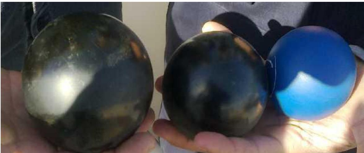
**Fig.Anx. 5:** Ball activated frac-sleeves.
