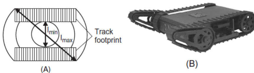
Figure I.18: (A) Illustration of the effective contact point and (B) a typical tracked platform
