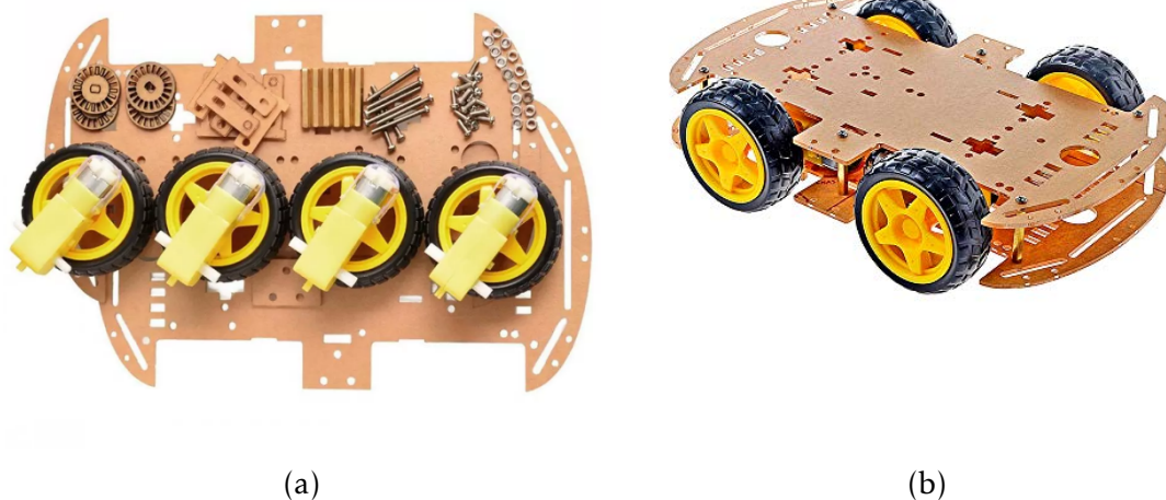
Figure III.21: (a)unassembled 4w Robotic Vehicle Chassis, (b) assembled 4w robotic vehicle chassis
