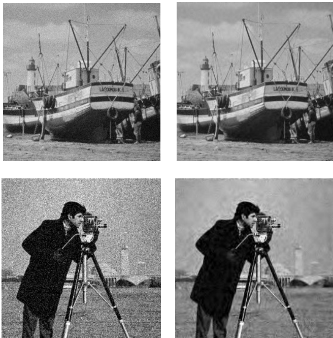
Figure 5. some gray scale image denoising using the proposed technique. (Left) Noisy image ( \sigma=25 ), (Right) proposed technique.
