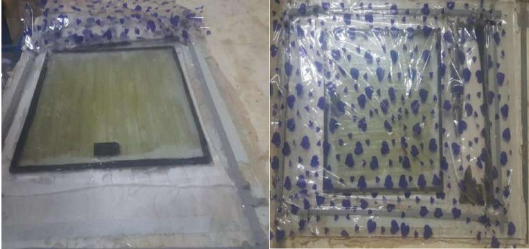
Figure III.5 Elaboration des plaques composites folioles de palmier dattier/polyester
