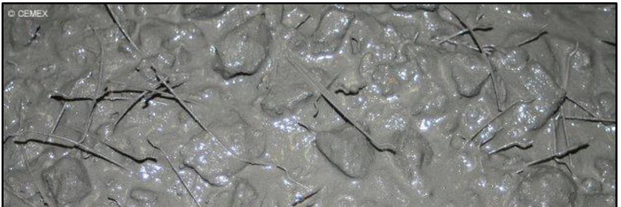
Figure I.5 : Béton fibré [3]
