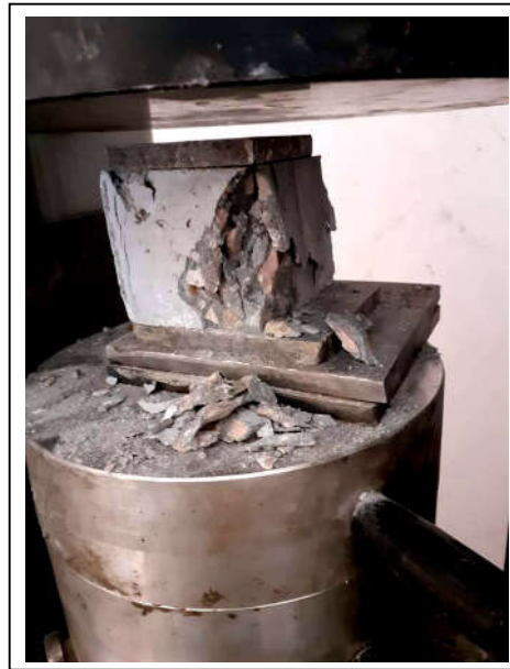
Figure III- 1: Essai de compression
