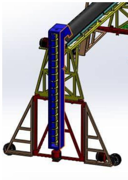
Figure III-25: Screw conveyor connected to the electrical motor
