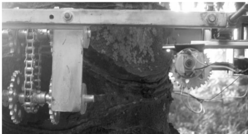
Figure II-9: Robot climbing smooth trunk using small sprockets [6]
