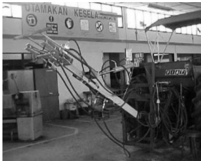
Figure II-6: Wire cutting mechanism mounted on tractor[6]
