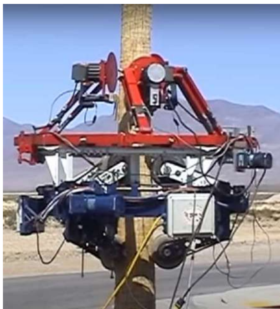
Figure II-11: Automated palm trimmer
