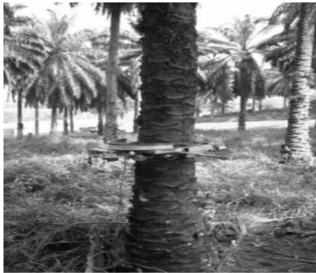
Figure II-8: Climbing robot with tilt sensors [6]
