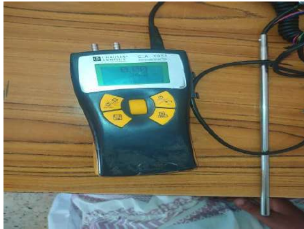
Figure (III.44) Velocity and temperature measuring device
