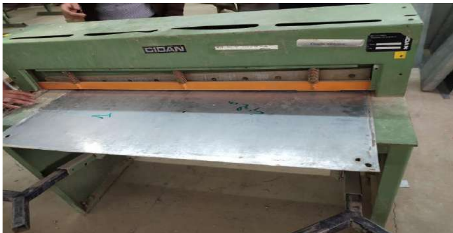
Figure (III.1) Guillotine shear
