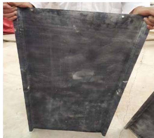
Figure (III.17.18) The folding process of the absorber (aluminum)
