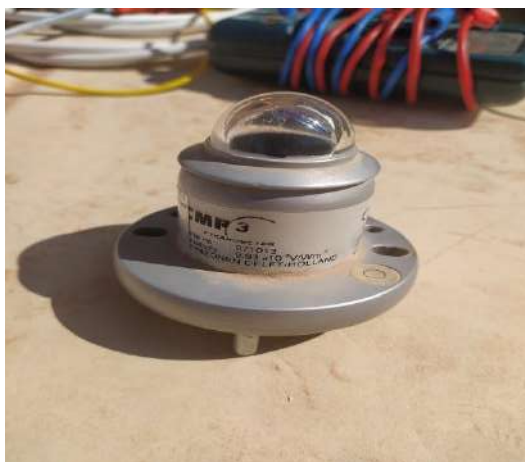
Figure (III.42) Pyranometre
