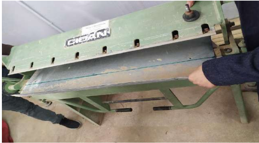
Figure (III.2) Universal sheet metal bending machine
