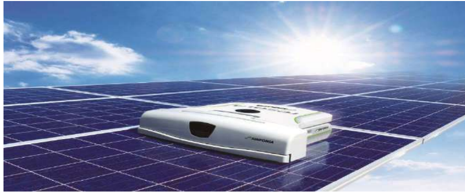
Figure (II-10): Robotic cleaning system (RCS).
