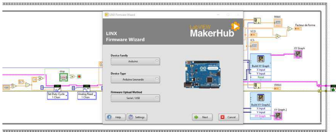
Figure (III-16): Linking LabVIEW and Arduino.
