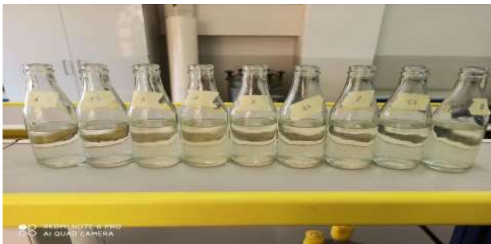
Les Figure N°22: Break point Chloration
