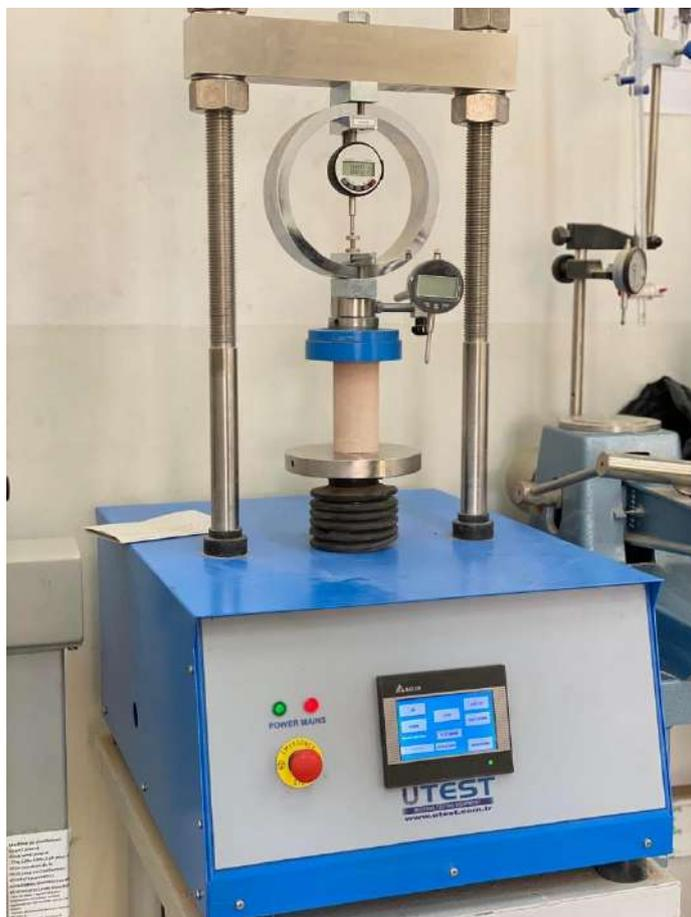
**Figure 15: machine de compression simple**
