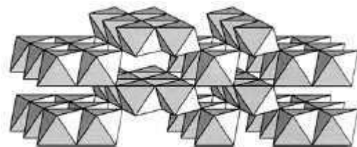
Figure I.5 Structure de la Nsutite [9].
