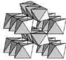
Figure I.3 Structure de la Pyrolusite [9].
