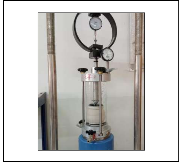
Figure 3.20: Clamping of the specimen in line with the perforated GTX
