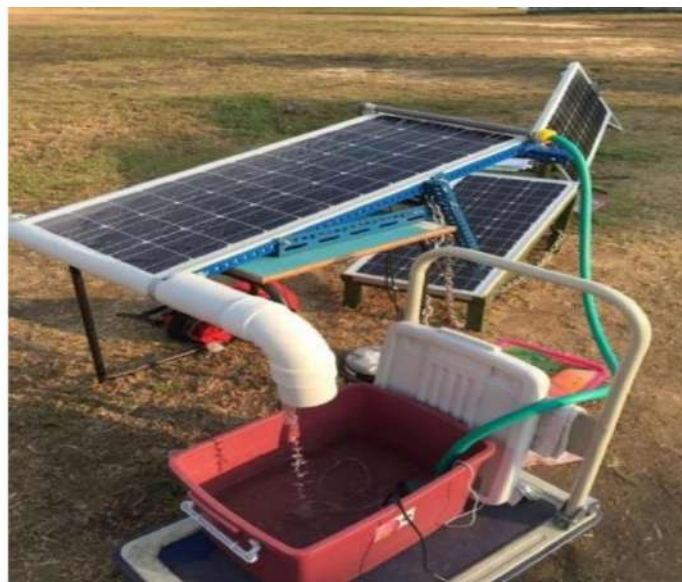
Figure II. 2: Experimental setup of cooling system [23]
