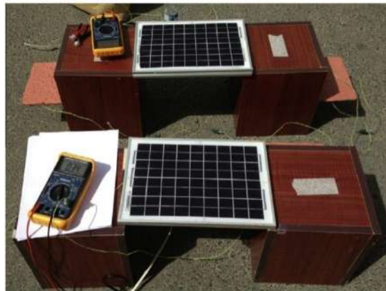
Figure II. 13: Experimental setup of cooling the PV module [31]
