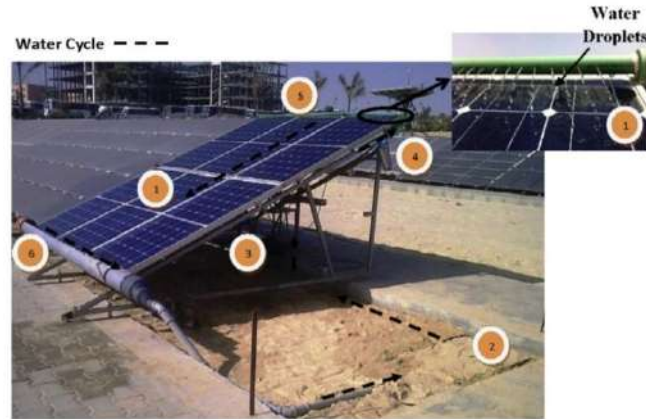
Figure II. 1: Experimental setup: 1.PV module, 2.tank, 3.pump, 4.filter, 5.nozzle and 6.drain pipe [22]
