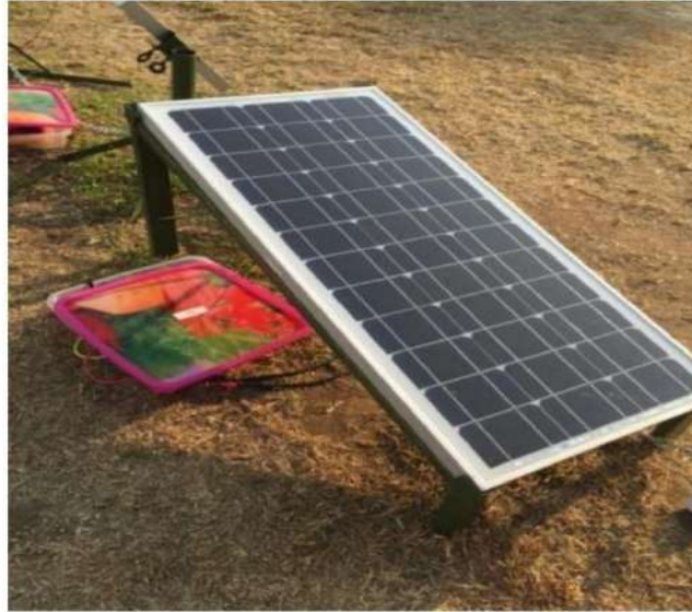
Figure II. 3: Experimental setup of non-cooling system [23]
