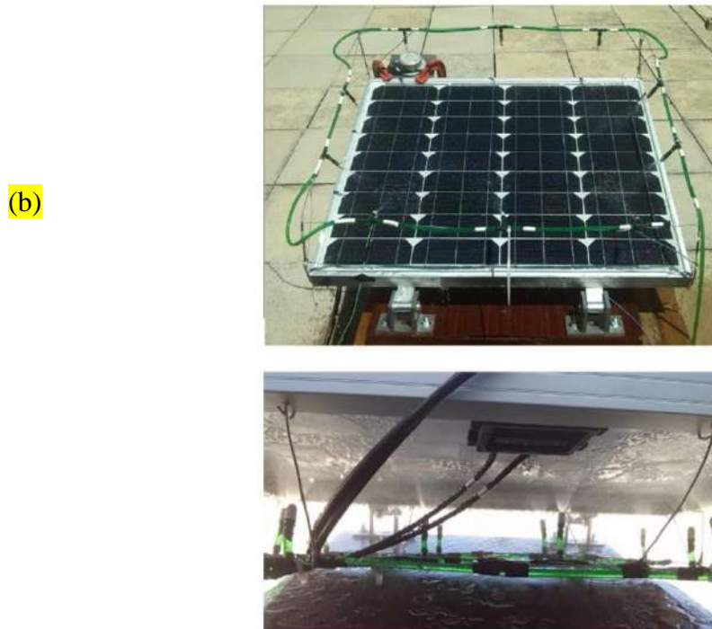
Figure II. 14: (a)Schematic layout of the specific experimental setup (b) The front and backside of the PV panel with the specific water nozzle system [40]
