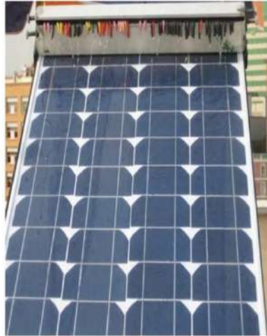
Figure II. 5: Front view of solar photovoltaic panel equipped with water film producer [25]
