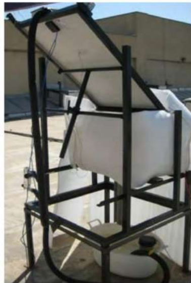
Figure II. 6: Pumping system and the heat exchanger of experimental combined Photovoltaic/Thermal (PV/T) system [25]
