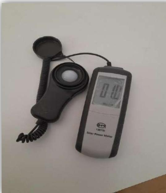
**Figure.IV.1** : solaremetre
