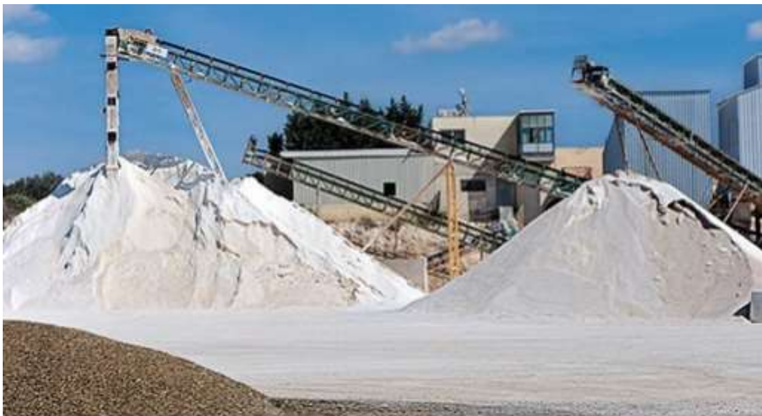
Figure (II.1): station de concassage.
