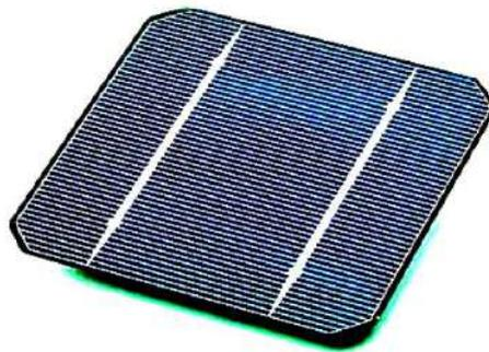
**Figure (1.20) :** Cellules monocristallines.
