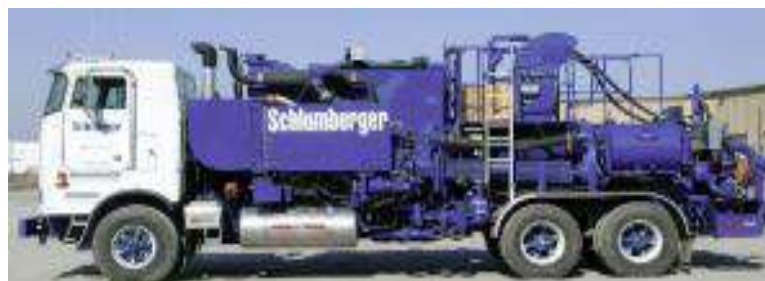
Fig 23: High pressure pumps
