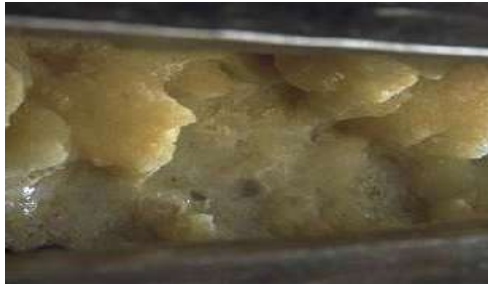
Figure I. 2: Calcium carbonates (CaCO 3 ) scale [4].
