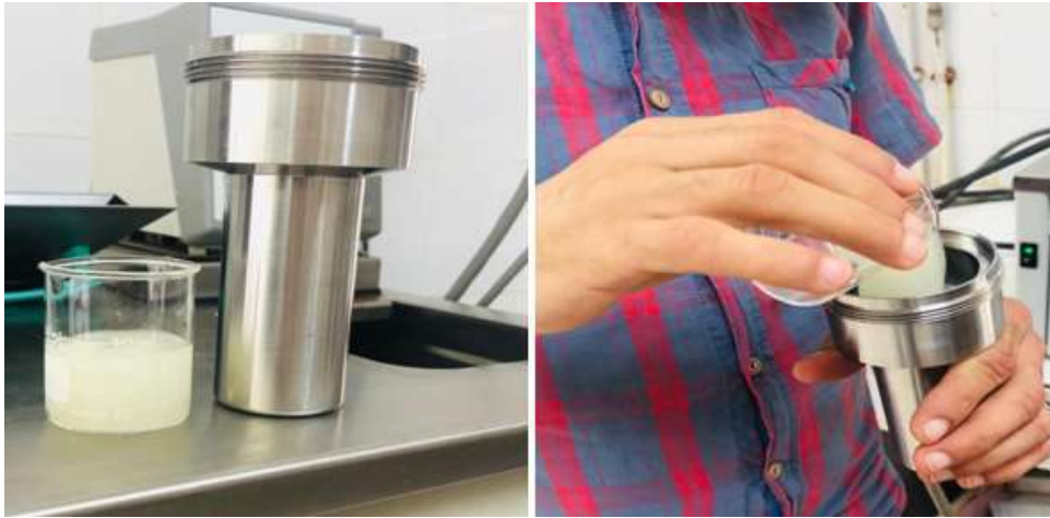
Figure III. 14: Viscosimeter cell with crosslinked gel.
