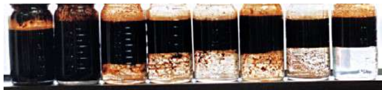
Figure I. 5: Emulsions with Crude Oil and Completion Fluids [5].
