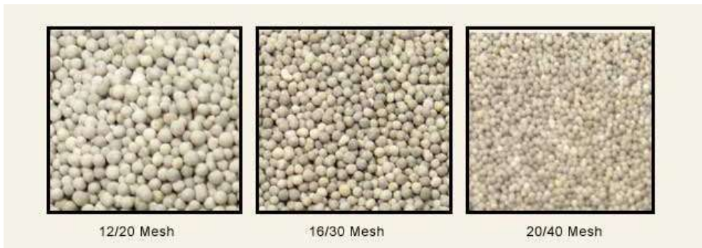
Figure I. 20: Different fracturing proppant size [18].
