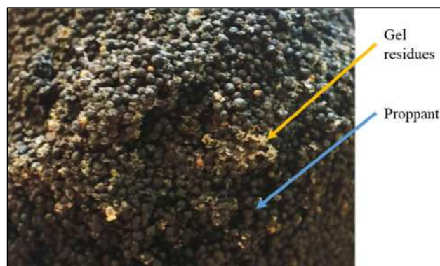
Figure III. 26: Gel residues after 24 h under 6000 psi at 120 °C with 5 lb/1000 gal breaker concentration.
