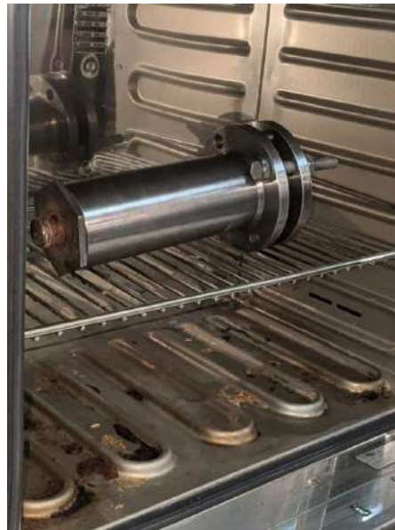
Figure III. 25: cell inside the oven at 120 °C.
