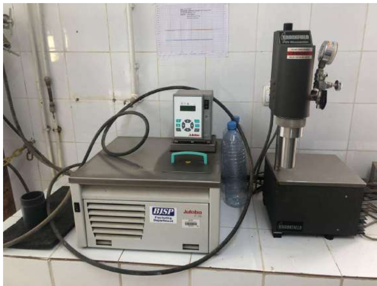
Figure III. 13: Measuring the viscosity of crosslinked gel with the rheometer.
