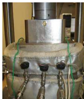
Figure II. 10: Experimental setup showing conductivity cell with heating jacket and pressure transducers [26].
