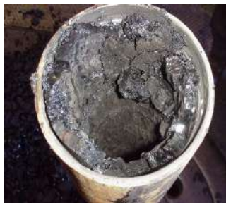
Figure I. 3: An example of an asphaltenes [4].
