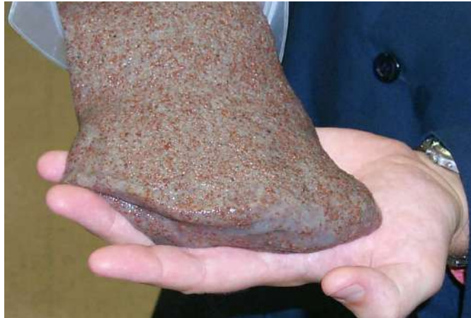
Figure I. 18: A Propped gel (Slurry) [9].
