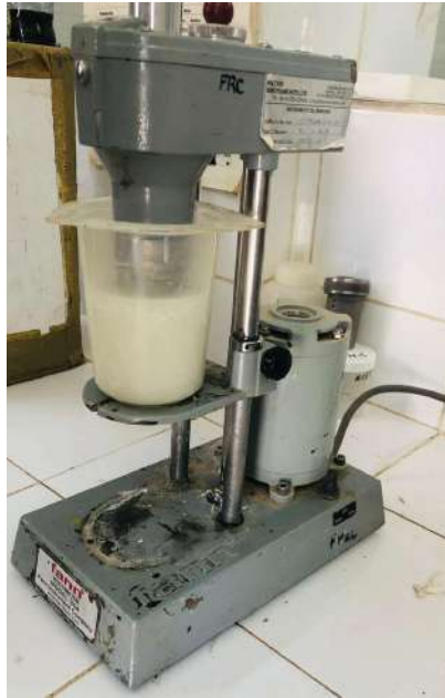
Figure III. 12: Measuring the viscosity of linear gel with Fann 35A.
