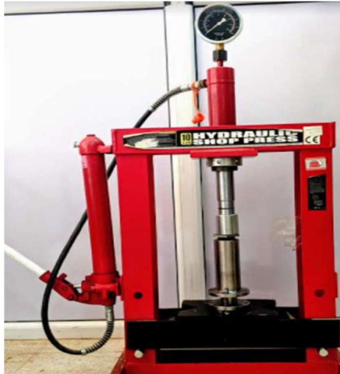
Figure III. 24: Applying pressure to the containment cell.
