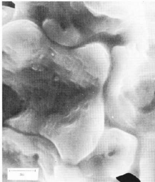
Figure III. 20: Guar polymer residue [47].
