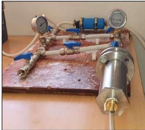
Figure II. 20: Installation schematic of the permeability measurement of proppant [37].
