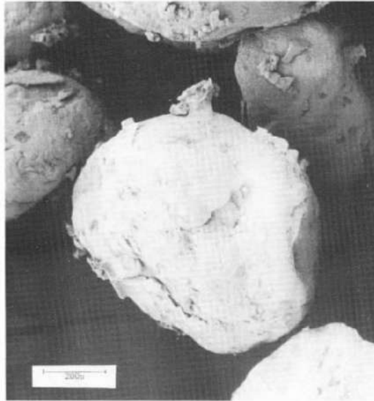
Figure III. 19: Sand grains covered with dried fracturing fluid residue [47].
