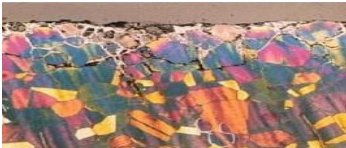
Figure II.4: Intergranular corrosion of stainless steel by HCl [21]
