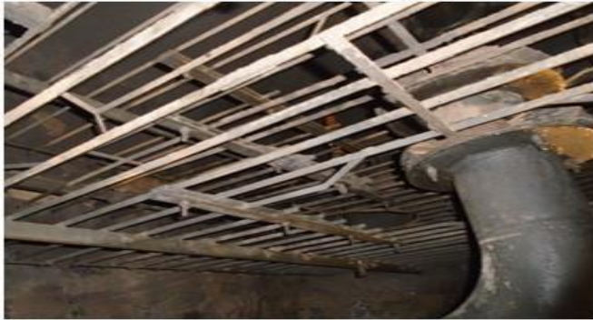
Fig.III..3:The horizontal grids in side Desalted (V-103 left,V-104 right)
