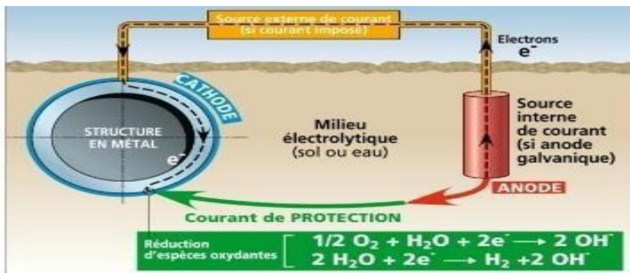
Figure II.6: Principle of cathodic protection [15]
