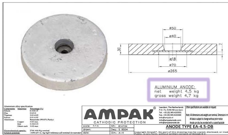
Fig .III.10.:Sacrificial Aluminum Disc anode which should be installed in Desalter [08]
