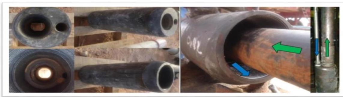
Fig.III.6 : double box Locator sub[9]
