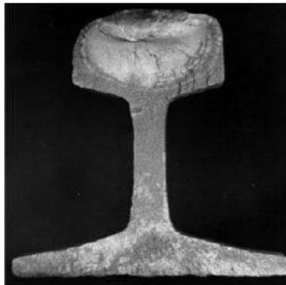
Figure I.32: Illustration 'Kidney-shaped' crack in rail head
