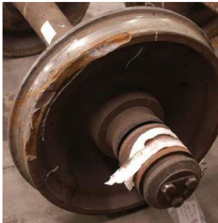
Figure I.46: Vertical Split Rim
