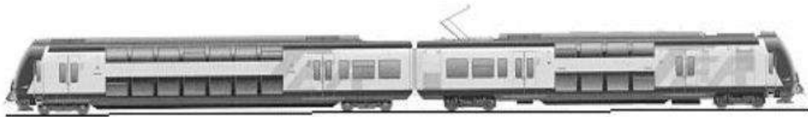
Figure I.9: Self-propelled Electric Multiple unit – EMU
